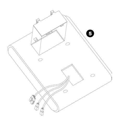
**5.** Load your console with the batteries provided. Batteries are 4 "AA" size.
